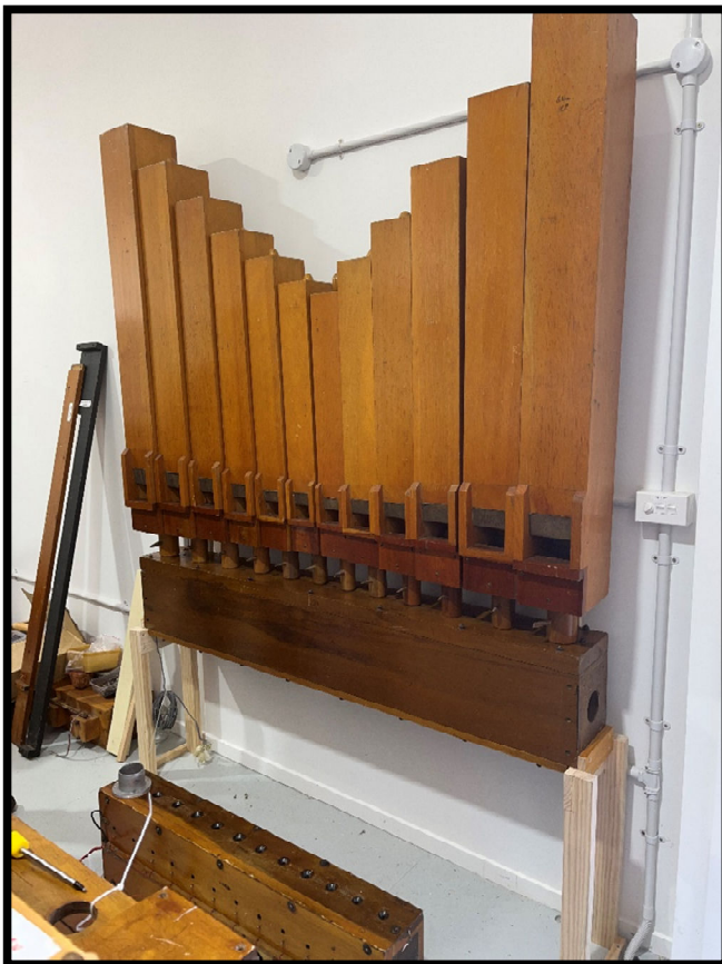
LEFT: Part of the Tibia rank of pipes. The Tibia is the foundation sound of the theatre organ and is rather like a big fat flute.
