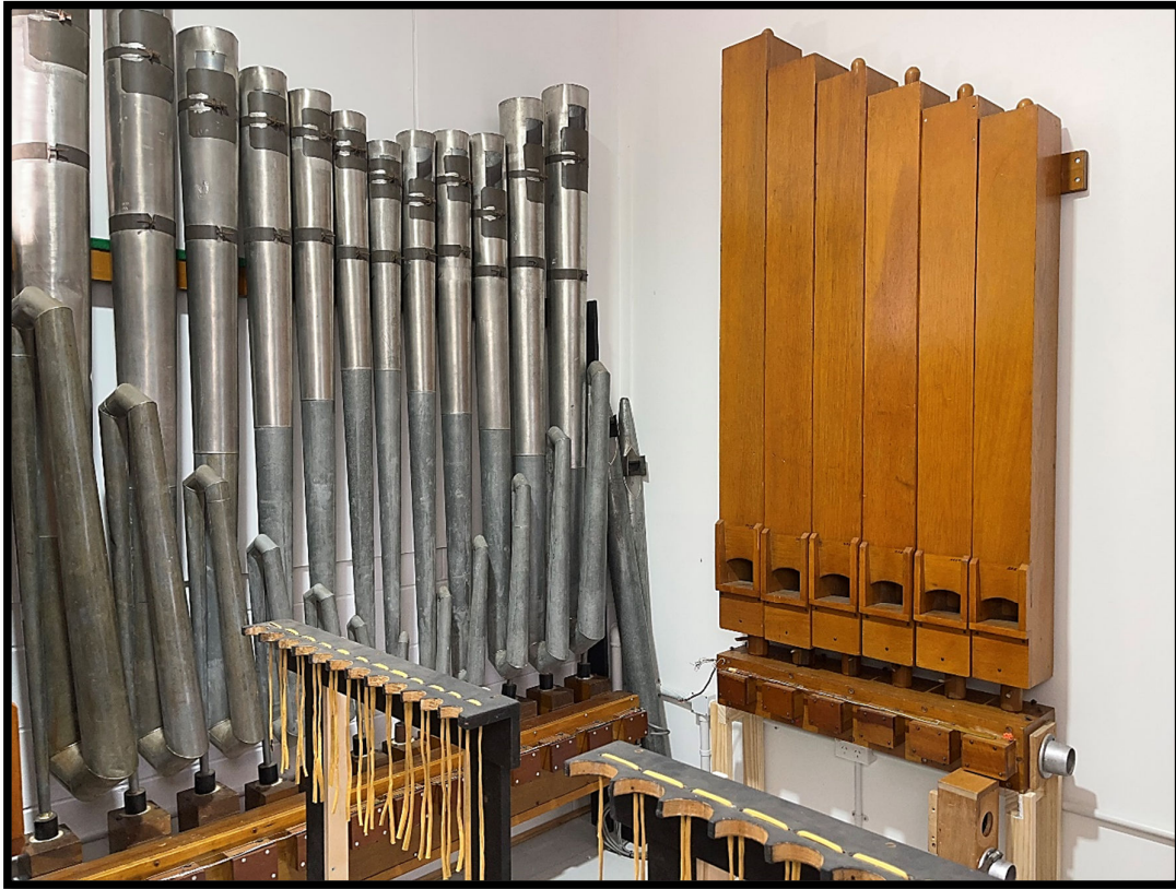
ABOVE: Main Chamber and the metal pipes of the Diaphone and part of the wood Bourdon. (Neil Warrington)
